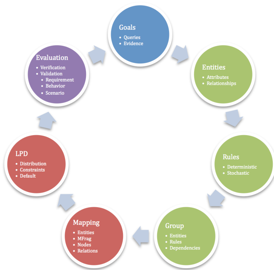
Figure 5.3: Probabilistic Ontology Modeling Cycle (POMC) - Requirements (Goals), Analysis & Design (Entities, Rules, and Group), Implementation (Mapping and LPD), and Test (Evaluation).
